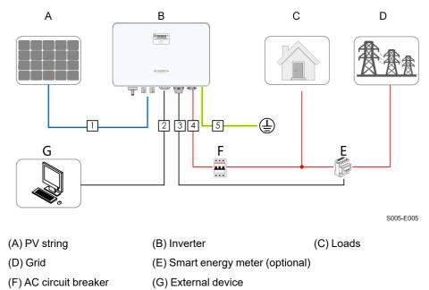
The electrical connection should be realized as follows(Includes optimizer):
