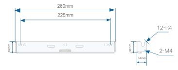
figure 4-1 Dimensions of Mounting-bracket
