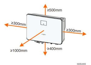
Install the inverter at an appropriate height for ease of viewing the screen and LED indicator and operating switch(es).
