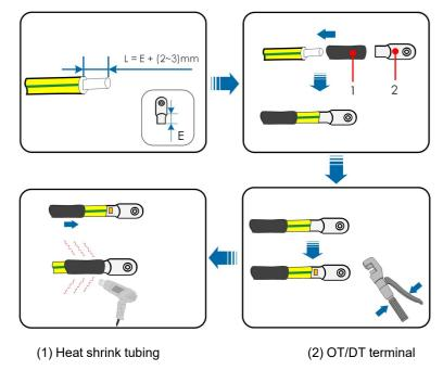
After being crimped, the OT terminal must wrap the wires completely, and the wires must contact the OT terminal closely.
