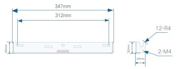
figure 4-2 Dimensions of Mounting-bracket
