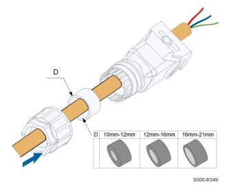
Step 3 Remove the cable jacket by less than 45 mm, and strip the wire insulation by 12 mm–16 mm.
