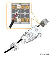
Step 6 Insert the terminal plug into the COM2 terminal at the bottom side of the inverter and then install the housing.
