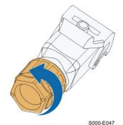
**Step 2** Thread the AC cable of appropriate length through the swivel nut, the sealing ring and the housing.
