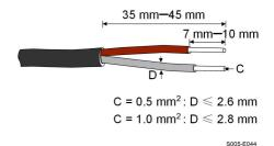
**Step 4** (Optional) When using a multi-core multi-strand wire cable, connect the wire head to the cord end terminal. In case of single-strand copper wire, skip this step.
