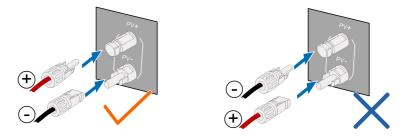
Step 3 Connect the PV connectors to corresponding terminals until there is an audible click.
