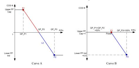
figure 7-18 Reactive Power Regulation Curve in Q(P) Mode
