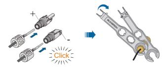
**Step 4** Check for polarity correctness.
