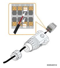
**Step 6** Insert the terminal plug into the **COM2** terminal at the bottom side of the inverter and then install the housing.
