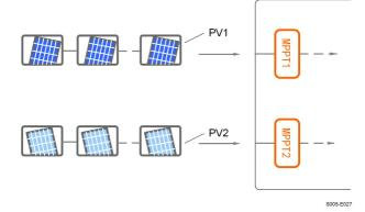
figure 5-3 PV Input Configuration (SG6.0RS for example)
