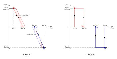
figure 7-19 Reactive Power Regulation Curve in Q(U) Curve
