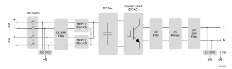
figure 2-5 Circuit Diagram (SG6.0RS for example)
